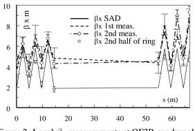
Figure 2: Local  $\beta_x$  measurements at QF2R quadrupoles.
