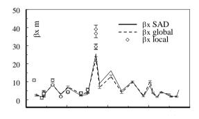
Figure 3: Global and local  $\beta_x$  values in the straight section.
