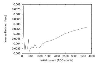
Figure 2: Inverse lifetime as function of the (initial) beam current in each interval.
