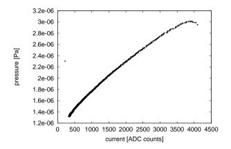
Figure 1: Measured average vacuum pressure in the ATF damping ring as function of the beam current.
