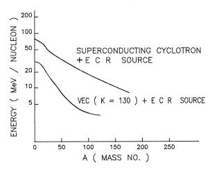
Figure 1: Energy /nucleon vs. mass for heavy ion beams to be available with VEC and superconducting cyclotron
