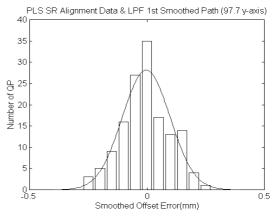
Figure 5. Histogram of the vertical displacements of quadrupole magnets in 1997.
