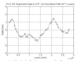
Figure 4: Vertical displacements of all storage ring magnets in 1997.
