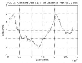
Figure: 2 Vertical displacements of all storage ring magnets in 1996.
