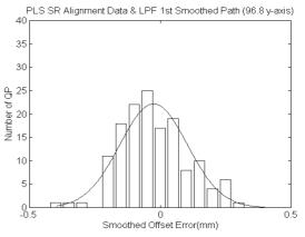
Figure 3: Histogram of the vertical displacements of quadrupole magnets in 1996.
