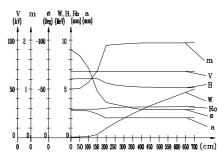
Fig.1: Main parameters of RFQ versus length
