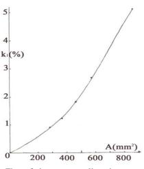
Figure3: k1 verse coupling slot area
