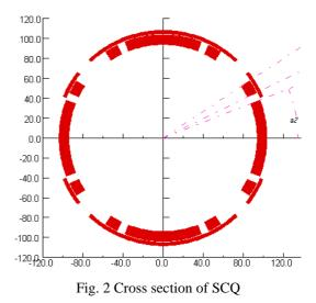
The SCQ coils are composed of quadrupole coil and vertical steering dipole coil. The quadrupole coil is a inner coil. The steering dipole coil is beside the quadrupole coil. The SCQ coils (both quadrupole coil and
