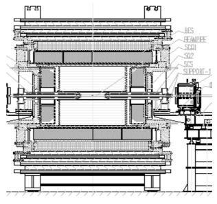
Fig. 8 Installation of BEPC-II IR Magnets
