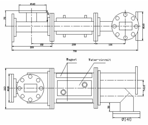
Fig.1 Differential phase-shift circulator
