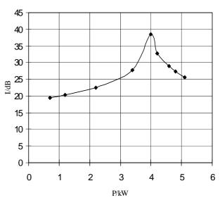
Fig.2 Isolation versus average power at F=2856MHz
