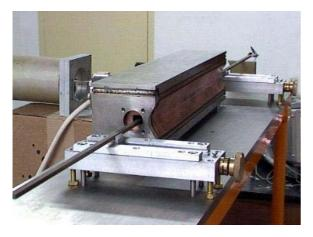
Fig. 2 The picture of the SSRF septum
