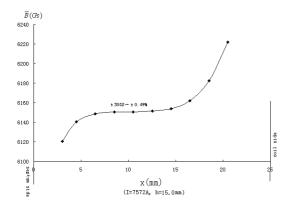
Fig. 6 The distribution curve of the main field
