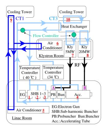
Fig. 1: Schematic diagram of the temperature control system and the measurement system. The letters A and B denote measurement points for the RF power and thephase. The numbers  $\underline{1}$  through  $\underline{10}$  are those for temperatures. The AC line voltage was also measured.
