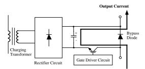
Figure 2(b): Cell-modulator when the switch is turned on.
