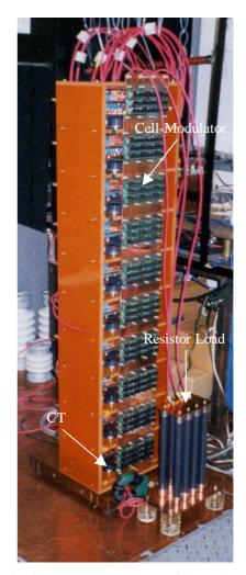
Figure 4: 10-stage test modulator with a resistor load.
