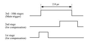
Figure 7: Trigger timing chart.
