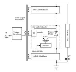
Figure 3: Simplified schematic of a 10-stage test modulator circuit.
