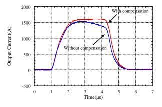
Figure 8: Output current waveform with and without compensation.
