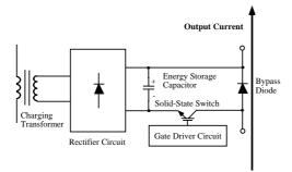
Figure 2(a): Cell-modulator when the switch is turned off.
