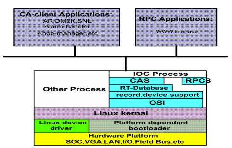
Fig.1: Software architecture of EPICS on Linux
