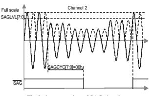
Fig.2. the generation of SAG signal
