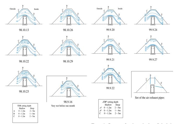
Figure 3: Contours of moisture in the soil bank in October 1998. It was rain of 25mm on October 21. These suggest that the water in the top of bank does not infiltrate to the bottom by the obstacle of the confined air above tunnel.
