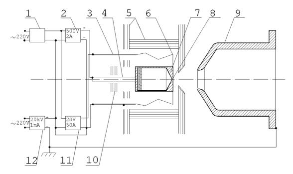
**Figure 3:** Ion source prototype schematic view. 1 - isolation transformer; 2 - direct current supply; 3 - cathode holder; 4 - container holder; 5 - thermal screens; 6 - cathode; 7 - container with graphite; 8 - emission hole; 9 - anode; 10 - additional thermal screen; 11 - cathode heater; 12 - accelerating voltage source.
