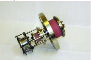
**Figure. 1:** *Picture of ion source prototype (side view)* The produced vapor which contains radioactive ions gets thermally ionized on the internal walls of a container. The flux of a mix of atoms and ions of radioactive elements is directed to the accelerating space via the
