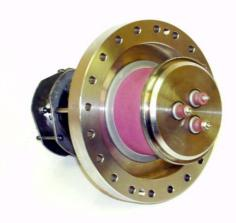
**Figure**. **2:** *Picture of ion source prototype (rear view)*
