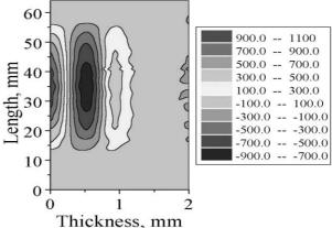
**Figure 3:** Distribution of tangential (above) and longitudinal (below) thermal stress (kPa) over the radial section of graphite for temperature distribution, presented in Fig.2
