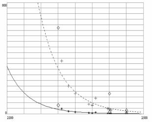
**Figure 4:** Dependence of samples lifetime (hours) on temperature ( $^{0}C$ ). • and O - measured values, + and  $^{0}$  - same values multiplied by factor 10, solid line - approximation, dashed line - approximate values multiplied by factor 10.
