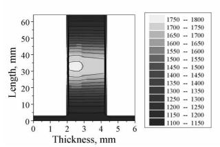
**Figure 2:** Temperature distribution over the section of graphite target in  ${}^{0}C$  for the graphite length 64 mm and disk thickness 1 cm
