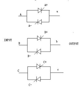
Figure 1: The main circuit of thyristor AC power controller
