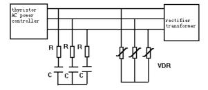
Figure 3: Improved low-frequency transient suppressor
