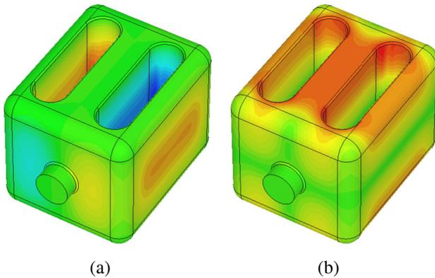
Figure 9: Surface (a) electric and (b) magnetic field of 400 MHz crabbing cavity.
