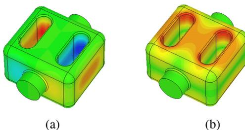
Figure 10: Surface (a) electric and (b) magnetic field of 800 MHz crabbing cavity.
