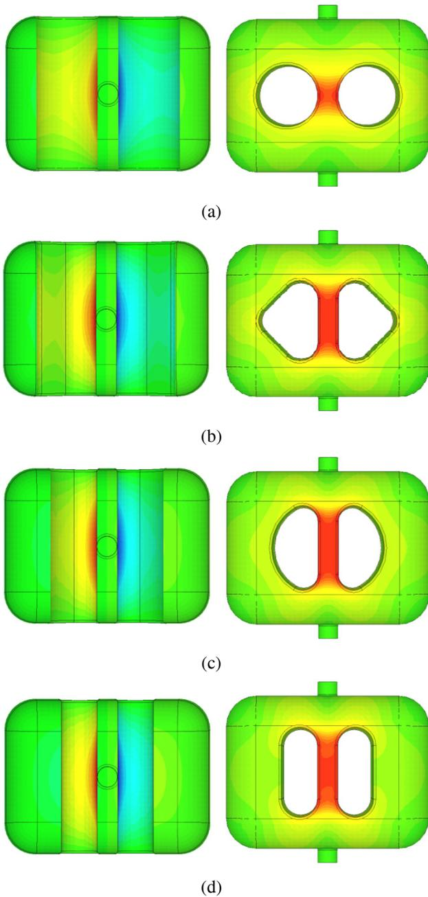
Figure 3: Surface electric field between the bars (left) and surface magnetic field on the top surface (right) of (a) circular, (b) triangular, (c) half circular and (d) race track shaped parallel-bar structures.
