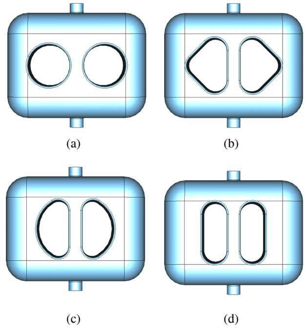
Figure 2: Design structures for CEBAF 499 MHz deflecting cavity with (a) circular, (b) triangular, (c) half circular and (d) race track shaped parallel bars.
