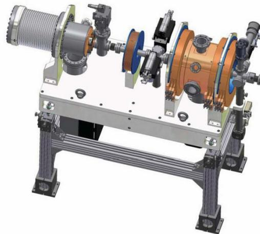
Figure 1: The NSLS-II linac front end produced by Research Instruments GmbH. [3]. The gun is on the left with the subharmonic buncher on the right.
