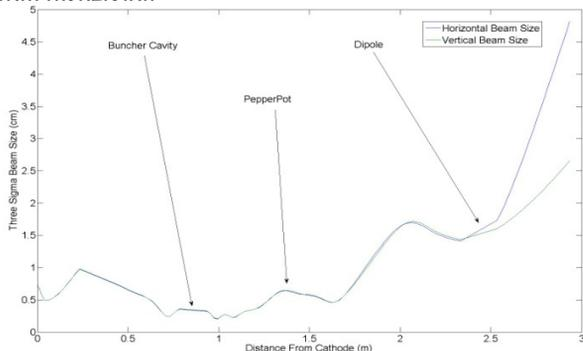
Figure 5: The three sigma beam size through the LFETS with the buncher turned on.
