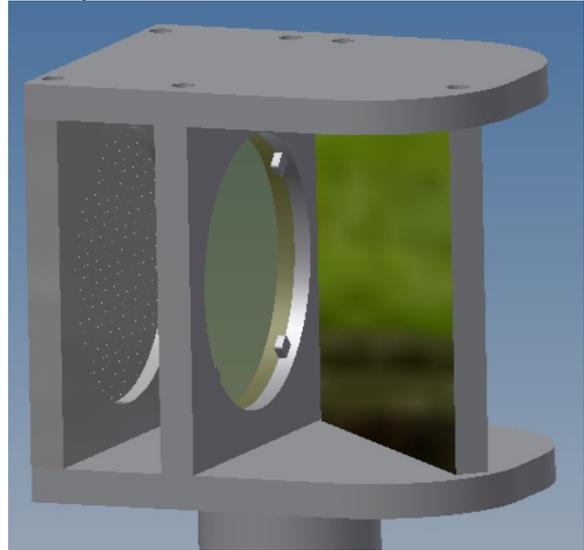
Figure 3: Conceptual Design of the pepper pot, florescent screen and 45 degree mirror assembly. The beam strikes from the left.
