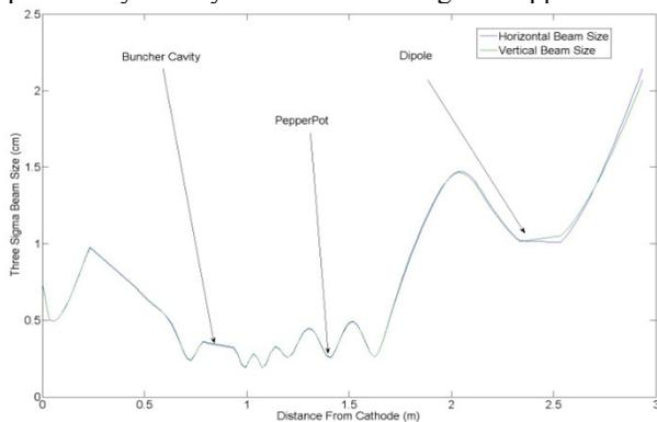
Figure 4: The three sigma beam size through the LFETS with the buncher turned off.
