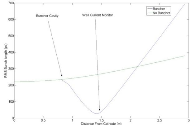
Figure 6: The rms bunch length through the LFETS with and without the buncher.
