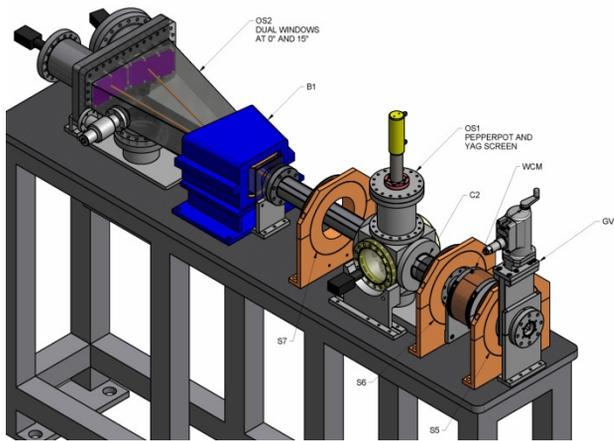
Figure 2: Conceptual design of the Linac Front End Test Stand. The LFE attaches at the gate valve on the lower right.
