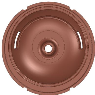
Figure 5: Solid model drawing of the cavity side of the end cell. The wall rounding was offset from the center axis compensate the perturbation in the magnetic field caused by the asymmetric slot geometry at the ends of the linac.
