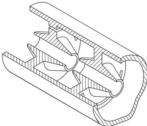
Figure 1: Slot resonance linac structure. Each slot extends nearly 180° in azimuth.
