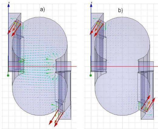
Figure 3: Slot modes of the DSRL with a) showing the lower frequency, symmetric mode and b) showing the higher frequency anti-symmetric mode.
