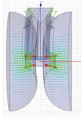
Figure 4: Accelerating mode of the DSRL. The electric field in the slot region is the parasitic coupling to the symmetric slot mode and results in RF losses. The anti-symmetric mode is unexcited.
