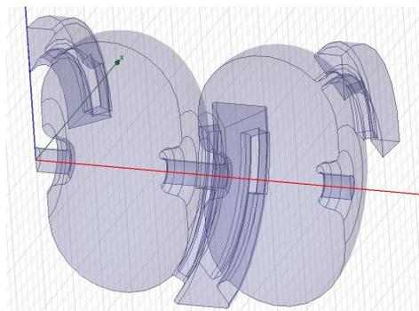
Figure 2: Dual slot resonance linac. Slots and void are not fully rounded in the HFSS model.
