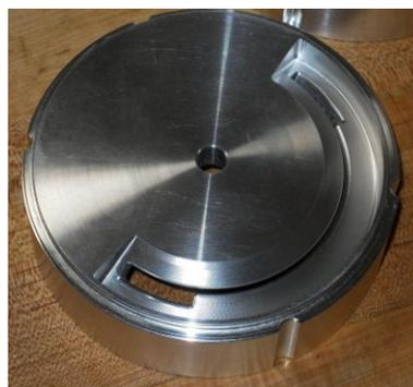
Figure 8: Void side of a machined DSRL half-cell.
