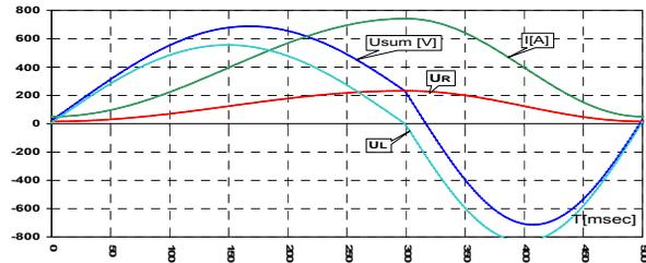
Figure 2: Current and voltage plots for 2Hz cycles for '1-cosine' shape of current ramps.
