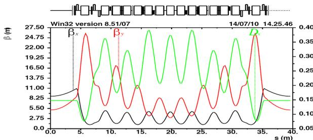
Figure 1: The betatron and dispersion functions for the lattice quadrant.
