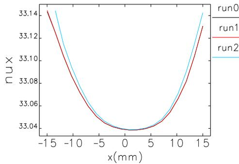
Figure 2: Amplitude-tune dependence at  $\delta = -2\%$
