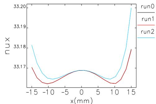
Figure 1: Amplitude-tune dependence at  $\delta = 0$
