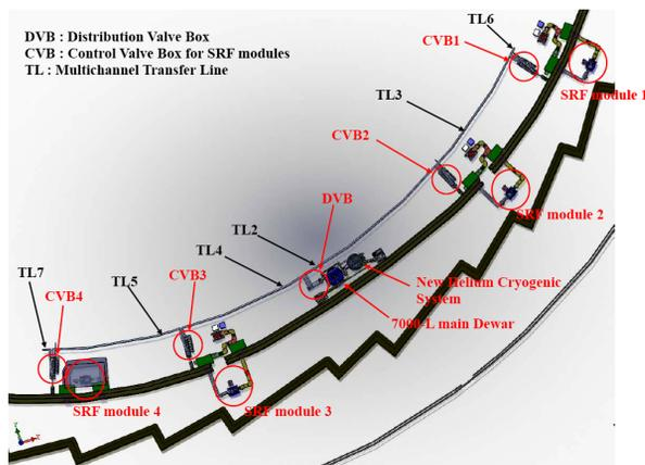
Figure 1: Overview of the layout of the new helium cryogenic system and the location of SRF modules.
