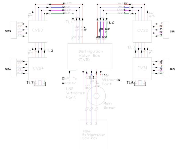
Figure 2: PFD of the transfer system.
