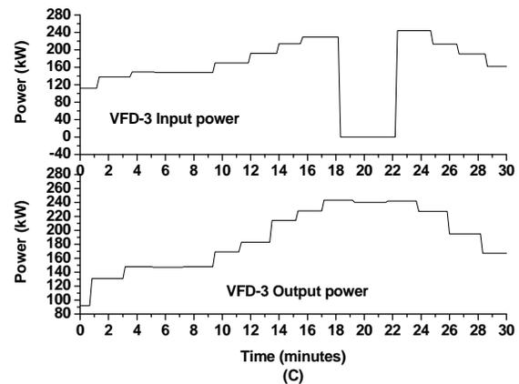
Figure 4: Test of the power capacity of the DC-Bank.
