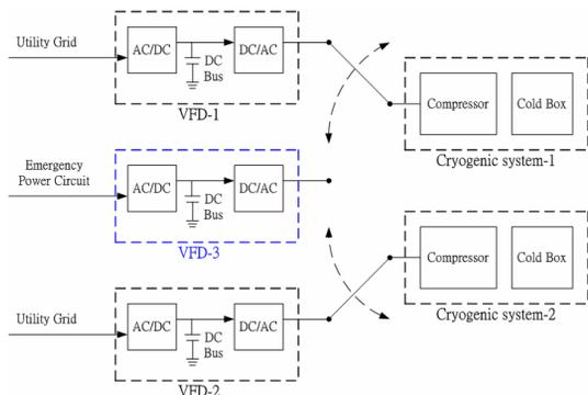
Figure 1: VFD back up function at NSRRC.
