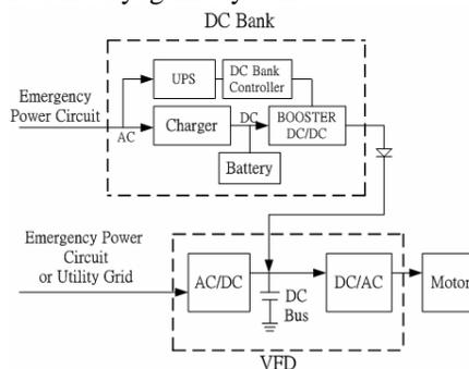
Figure 2: Configuration of the DC-Bank system.
