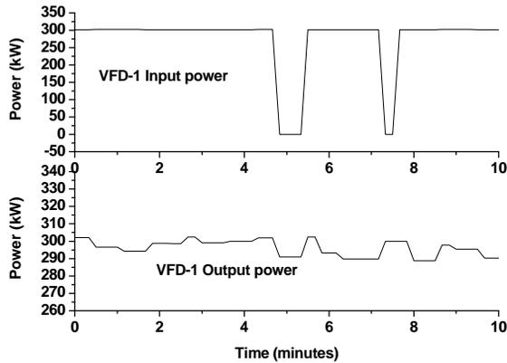
Figure 5: Test of power sag of the DC-Bank.
