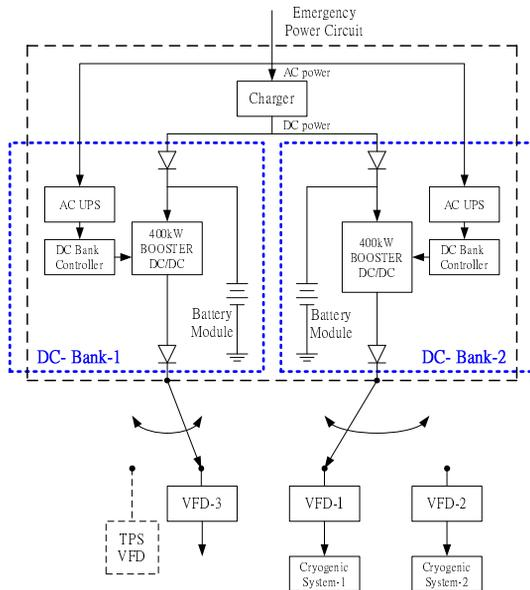
Figure 3: Configuration of the cryogenic system with the DC-Bank at NSRRC.
