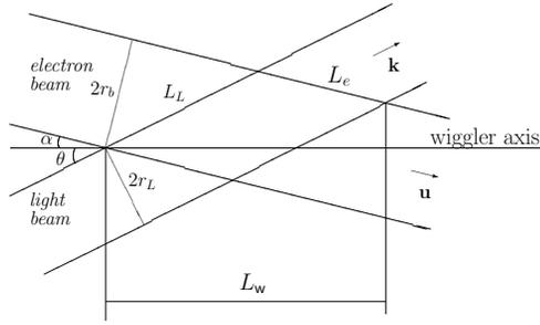
Figure 1: The scheme in  $xz$ -plane of undulator with non-collinear arrangement.
