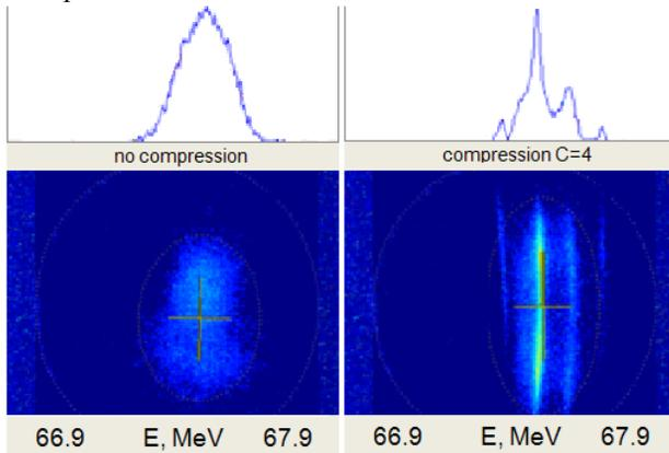
Figure 3: Spectra of uncompressed (left plot) and compressed (right plot) beams.
