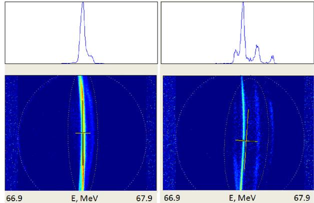
Figure 4: Compressed beam with the chirp removed by tank 3 at spectrometer (left plot) and zero phasing measurement performed with tank 4 (right plot).
