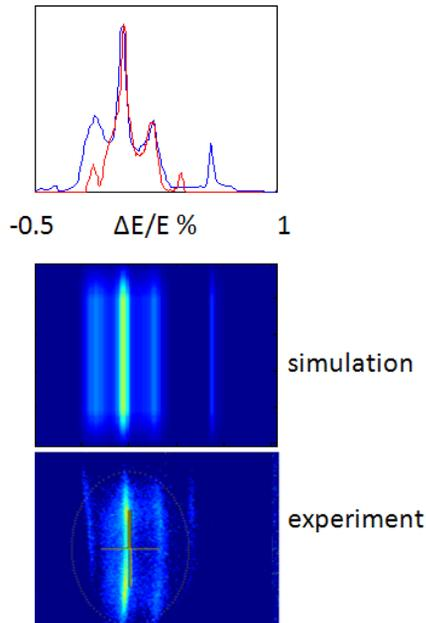
Figure 5: A comparison of the simulated (blue) and the measured (red) spectra of compressed beam.
