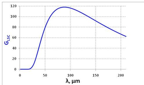
Figure 2: LSC-driven microbunching gain at SDL.
