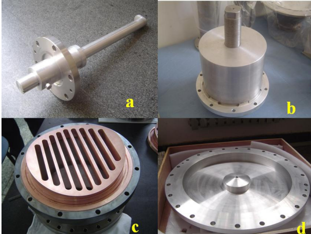
Figure 6: Aluminum cold models: postcoupler (a), slug tuner (b), vacuum grill(c), end wall (d).
