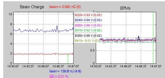
Figure 9: Time records of beam charge, laser energy and BPMs intensity.
