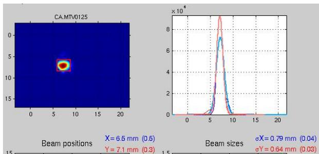
Figure 4: Laser pulse on the virtual cathode after shaping.
