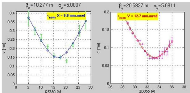
Figure 8: Horizontal and vertical transverse Twiss parameters reconstructed from quadrupole scan.
