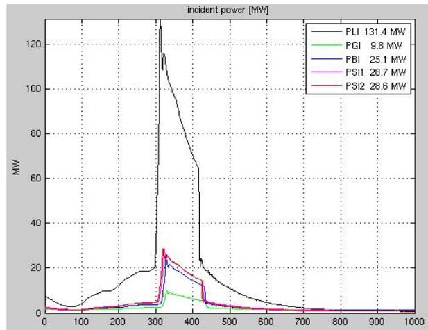
Figure 5: Power after pulse compression: *PLI*, at gun input; *PGI*, at buncher input; *PBI*, at accelerating structures inputs; *PSII* and *PSI2*
