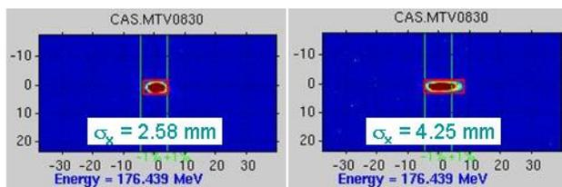
Figure 7: energy spectrum with 12 GHz CLIC structure switched OFF (left) and ON (right) at zero crossing.
