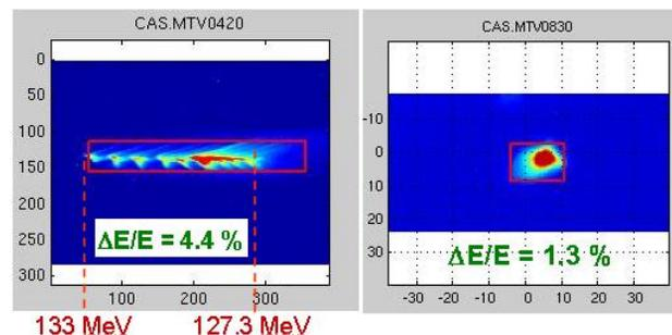
Figure 6: Energy spread for a pulse of 10 bunches. Laser timing vs. RF pulse governs its value.
