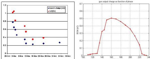
Figure 3: evolution of QE and of bunch charge during 6 weeks and gun RF phase scan.
