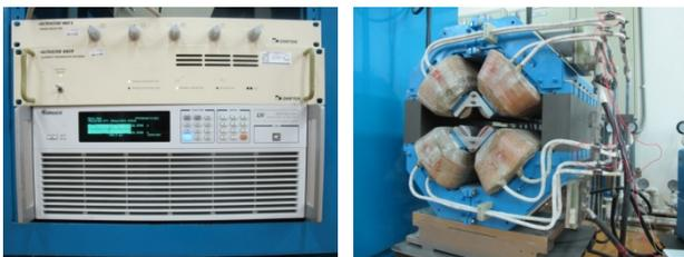
Figure 2: Quadrupole power supply and quadrupole magnet loading at laboratory.
