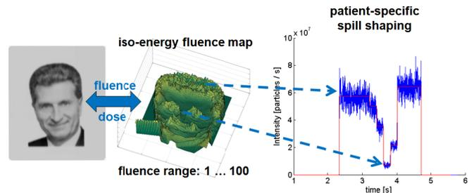
Figure 2: Patient-specific dynamic spill shaping will be driven by the particle fluence definition which is the result of the treatment planning process. This teaching example shows dose distribution (raster scanned portrait, left) and the corresponding fluence map (center). The high-dose parts (upper arrow) will be irradiated using the high-intensity part of the spill structure (right). Whereas the low-dose parts require the extraction of low intensities (lower arrow).
