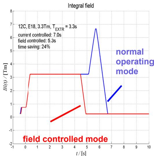
Figure 1: Magnetic field feedback relevantly reduces the cycling time of the HIT synchrotron as the extraction can be started earlier and the ramping to the maximum field level is no longer needed.
