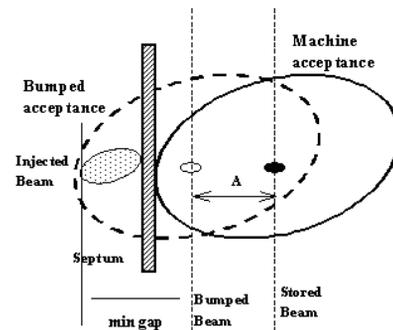
Figure 2: The schematic diagram of injection.
