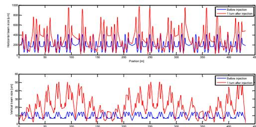
Figure 8: The beam profile before and after injection using PQM.
