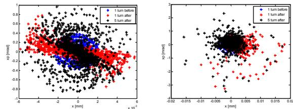
Figure 7: The beam before and after injection using PQM and PSM.
