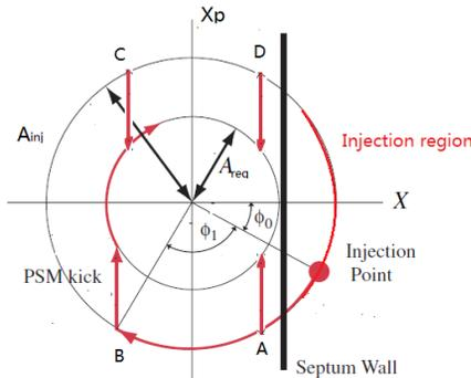
Figure 3: A trajectory of an injected beam in PSM injection on a normalized phase space [3].
