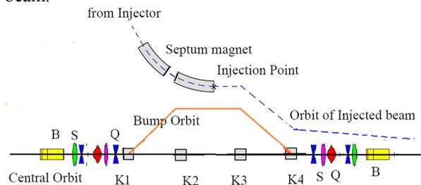
Figure 1: The injection scheme of SSRF.
