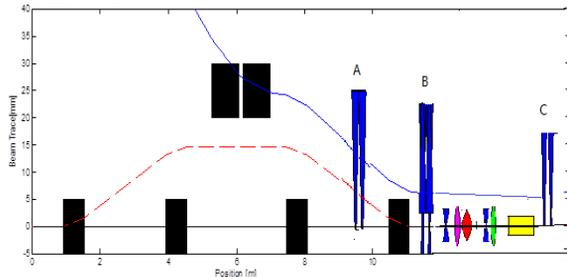
Figure 5: The Injection scheme of PM and four-kicker bump.
