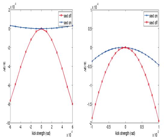
Figure 1: Beam energy changes with a horizontal kick in dispersion-free region. In NSLS-II ring (left) the cancellation is quite accurate (see blue curve), but for the small NSLS-VUV ring (right), the cancellation not so perfect (blue curve).
