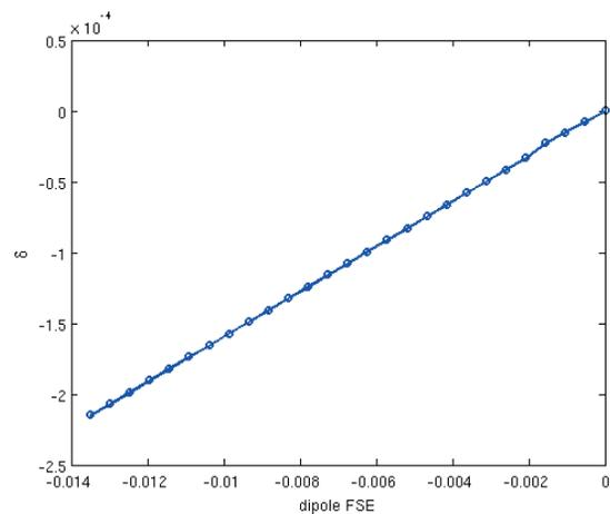
Figure 3: Beam energy change with a single dipole field loss without orbit correction.
