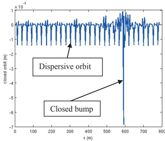
Figure 4: Closed bump to compensate the shorted dipole and dispersive orbit due to beam energy change.
