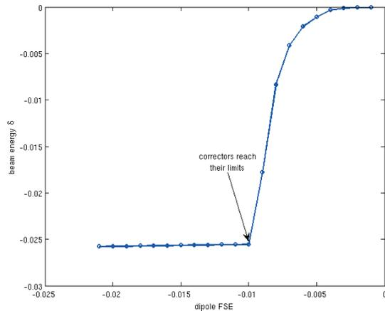
Figure 6: Beam energy change with orbit correction to compensate a shorted dipole. Beam energy change stops once corrector magnets are saturated.
