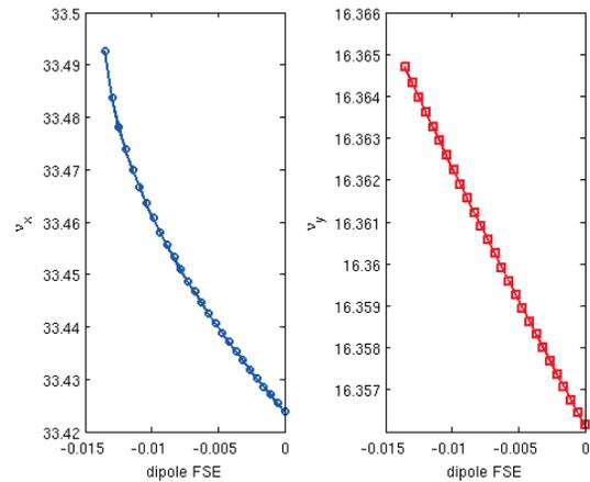
Figure 2: Beam tune-shifts with a single dipole field loss without orbit correction.
