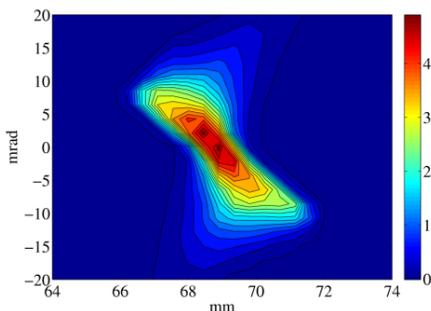
Figure 2: Phase space as mapped by the Allison emittance scanner, for a 60 keV, 10 mA peak electron beam. The normalized r.m.s. emittance is 4.6 microns.
