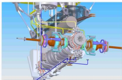
Figure 3: Injector cryomodule internal assembly.
