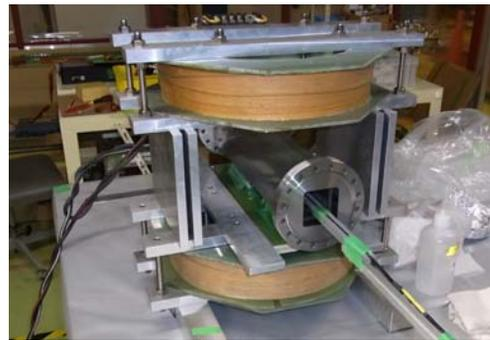
Figure 3: Setup of the magnetic field measurement with the 1-dimensional Hall probe.
