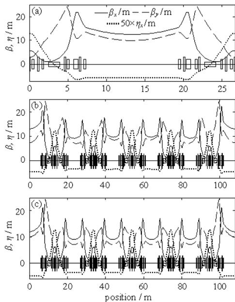
Fig. 4: Linear optics design of the low- $\alpha_C$  optics in the SSRF storage ring.
