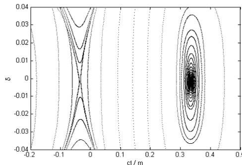
Fig. 6: Longitudinal phase map of the SSRF storage ring with a low-negative  $\alpha_C$  optics
