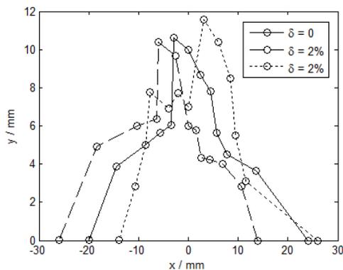
Fig. 5: Dynamic aperture (injection point) of the SSRF storage ring with a low-negative  $\alpha_C$  optics
