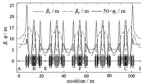
Fig. 1: Lattice layout and nominal linear optics in one fold of the SSRF storage ring
