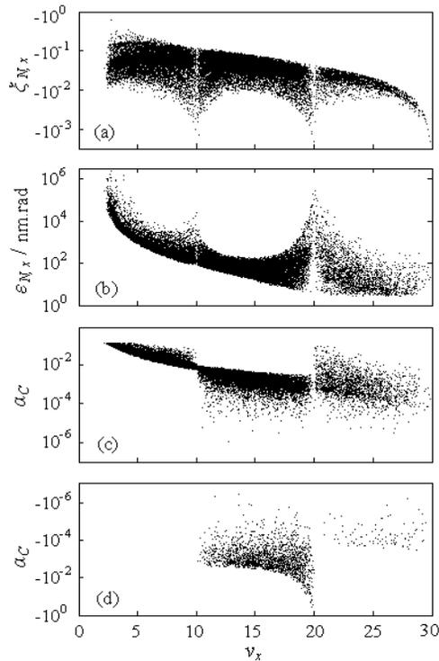
Fig. 2: Beam parameters as a function of the horizontal tune, (a) is the natural horizontal chromaticity, (b) is the natural emittance, (c) is positive values of the momentum compaction factor, and (d) is negative ones
