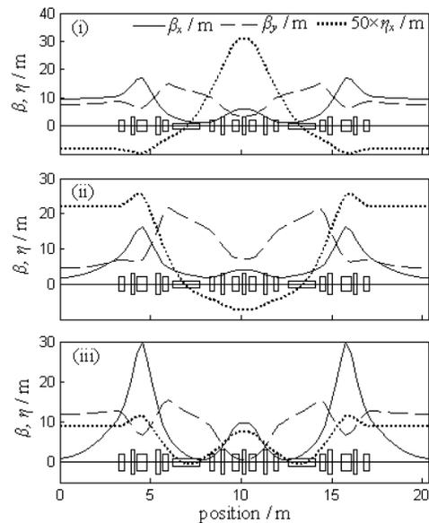
Fig. 3: Three low- $\alpha_C$  optics in one cell of the SSRF 20-cell-periodic lattice.
