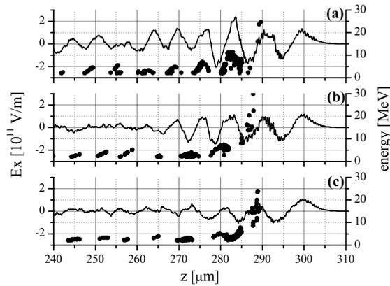
Figure 4: One dimensional PIC results with different density structure. (a) shows the acceleration field strength (solid line) and particle energy (dot) for the uniform density case with plasma density  $2.2 \times 10^{19} \text{ cm}^{-3}$ . (b) for the density change slope was  $6.7 \times 10^{15} \text{ cm}^{-3}/\mu\text{m}$ , and (c) for  $2.3 \times 10^{16} \text{ cm}^{-3}/\mu\text{m}$ .
