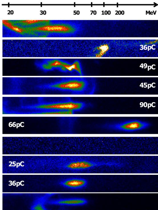
Figure 2: Electron beam energy and charge for 10 consecutive shots. The energy of the beam position is shown in the top bar. The bunch charge is shown in each beam image in white character.
