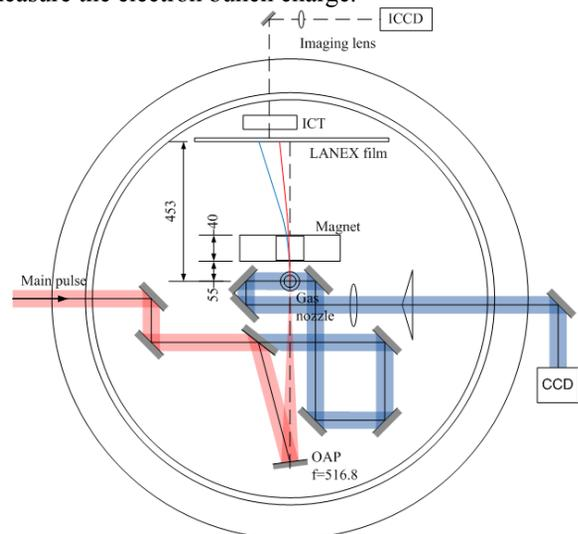
Figure 1: Experimental setup. Red and blue bar shows the direction of the main laser pulse and the probe beam for the interferometer. The laser pulse was focused using off axis parabolic mirror with 516 mm focal length. Just after the nozzle, a permanent magnet was used to bending the electron beam path with respect to the beam energy. The distance from the gas nozzle to the Lanex screen is 450 mm.
