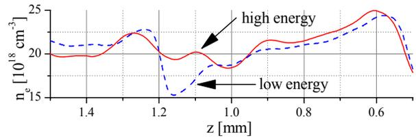
Figure 3: Plasma density structure for low(dashed line) and high energy(solid line) case. The zero position is at the edge of the nozzle. The laser pulse propagates along the z direction(from right to left in the graph).
