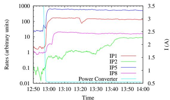
Figure 1: First collisions as seen by the BRANs in all IPs. The power converter data illustrates the moment when the injection separation bumps were ramped down.
