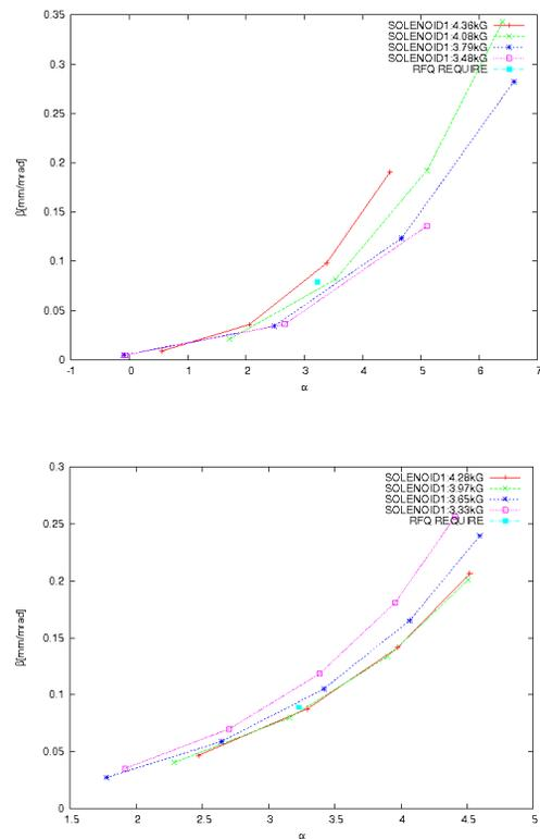
Figure 4: The PBGUNS-simulated tuning curves with variation of axial magnetic field strength. Conventional solenoid magnet (above) and hybrid solenoid magnet (below).
