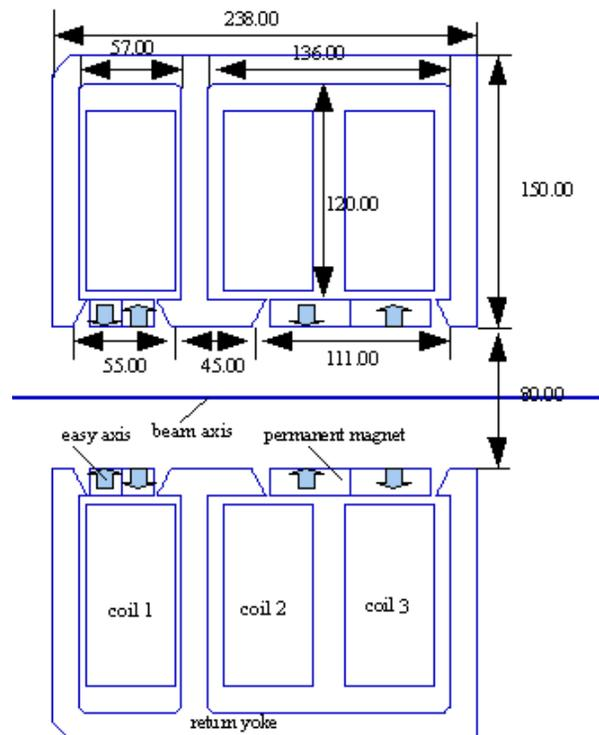
Figure 2: Cross section of the hybrid solenoid coil.
