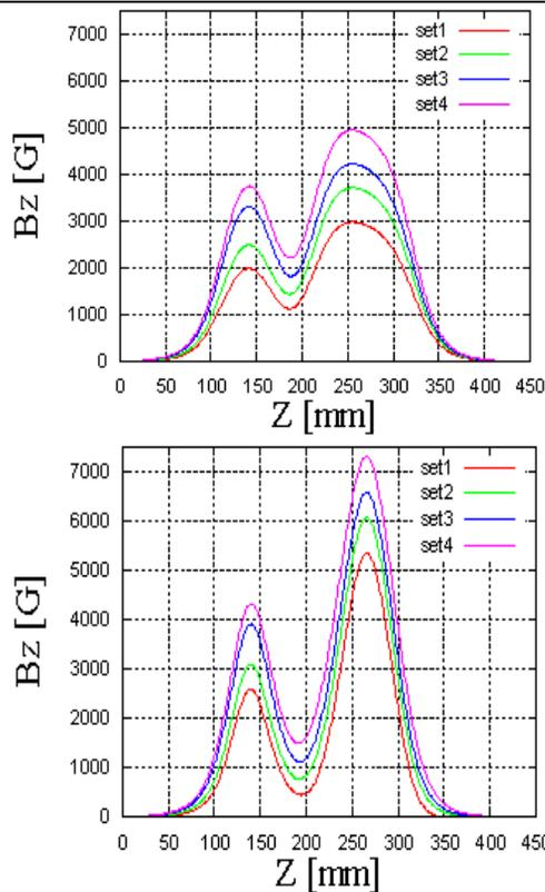
Figure 3: Magnetic field distribution. Conventional solenoid (above) and hybrid model (below).
