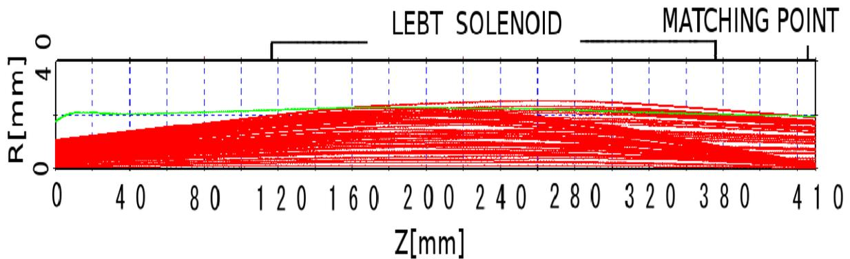
Figure 6: Trajectories in LEBT simulated by PBGUNS
