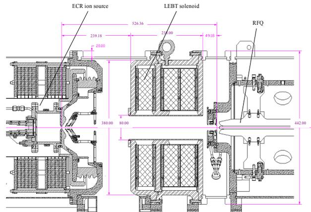
Figure 1: Schematic of ECR ion source, LEBT, and entrance of RFQ.
