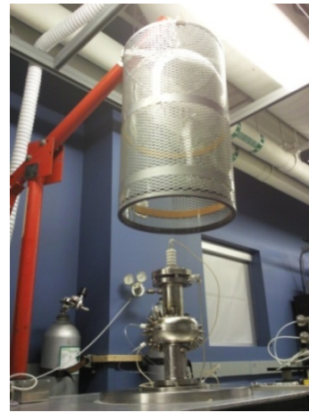
Figure 4: Bell jar system for single cell cavity with multiple optical fiber diagnostic setup
