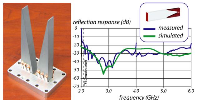
Fig.6. Broadband low-power HOM load prototype.
