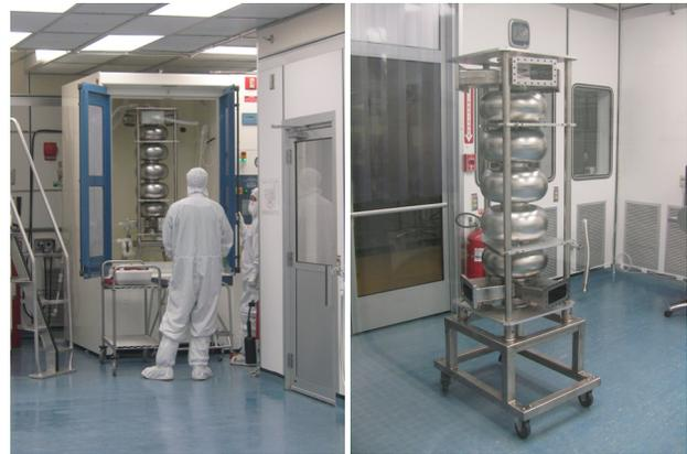
Fig. 4. 750 MHz high-current cavity in preparation.
