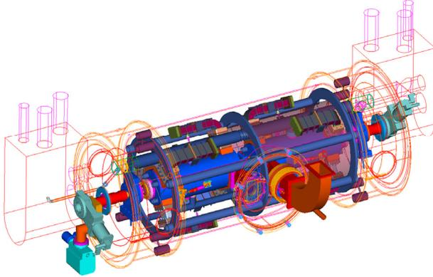
Fig. 7. Concept for a high-current test cryounit.
