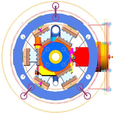
Fig.8. Cross section of high-current test cryounit showing helium circuit, space frame and support rods.
