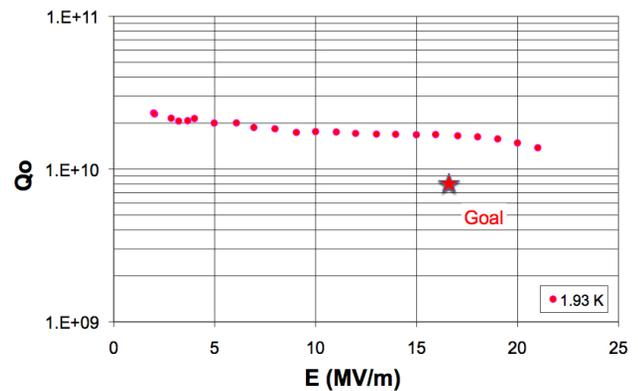
Fig. 5. First test result of 750 MHz five-cell cavity.
