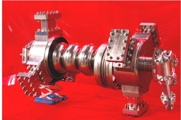
Fig. 1. 1.5 GHz 5-cell high-current cavity ready to test.
