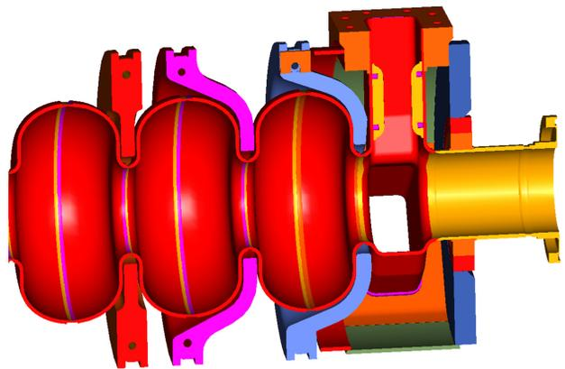
Fig. 2. Standard and offset tuning plates for the HC cavity.
