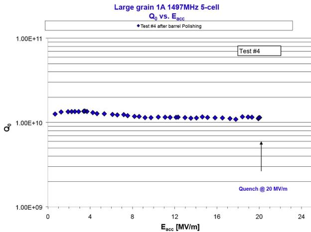
Fig. 3. Test result of 5-cell 1.5 GHz cavity after CBP.
