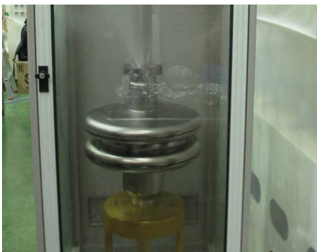
Figure 3: High pressure rinsing of the cavity.
