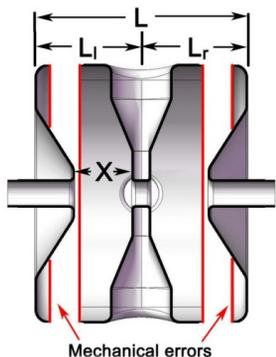
Figure 7: The major mechanical errors in the considered region of PKU SSC.
