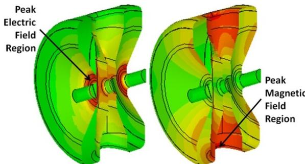
Figure 2: Surface electric (left) and magnetic (right) fields in PKU SSC. The field strength increases as the color changes from green to red.
