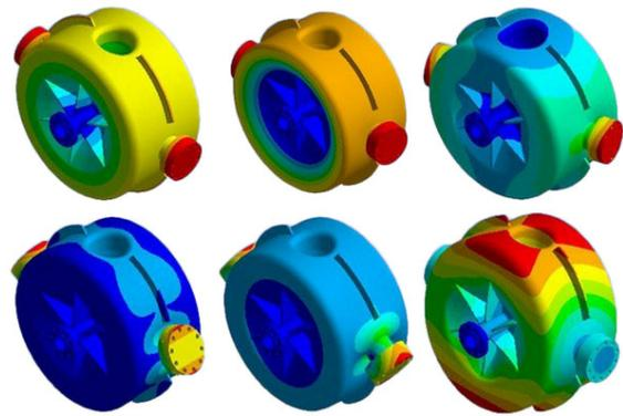
Figure 5: The total deformations of the lowest six mechanical resonance modes. The deformation is increased with the colour changing from blue to red.
