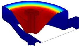
Figure 4: The displacements of cavity tuning. All the deformation occurs at color changing region.
