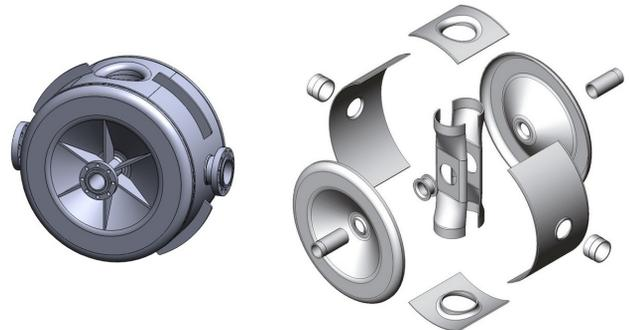
Figure 6: The stiffening ribs structures of PKU SSC, and the divided components without stiffening ribs and flanges.
