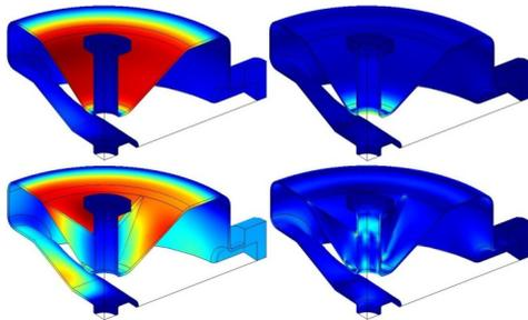
Figure 3: The SSC deformation and von mises stress under 1atm external vacuum load. (left) deformation; (right) von mises stress;(top) without stiffening ribs; (bottom) with stiffening ribs.
