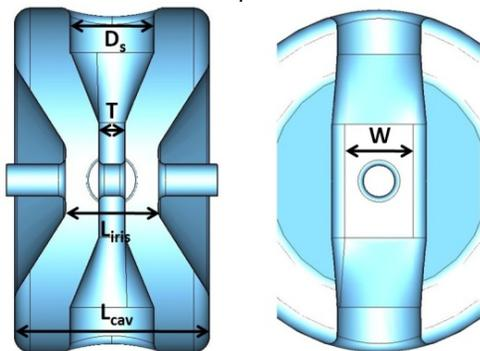
Figure 1: Cross section of the PKU SSC with the main parameters used in the optimization.
