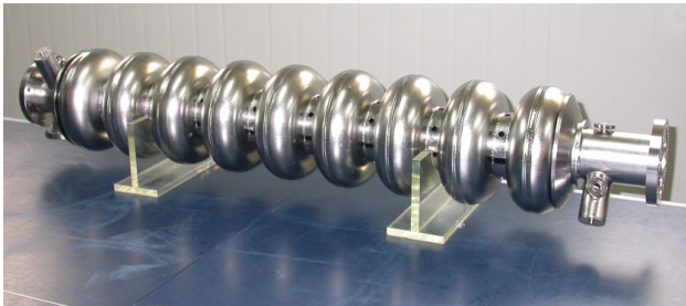
Figure 1: The home-made 9-cell TESLA type cavity.
