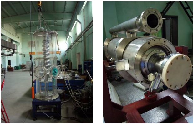
Figure 3: The glove box, and the seams to be welded
