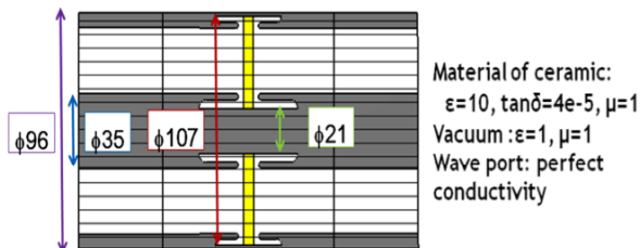
Figure.4: Calculation model of the ceramic window. The detailed initial parameters of ceramic window are shown.
