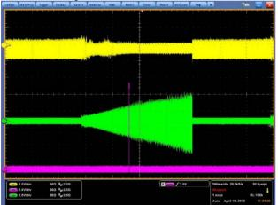
Figure 2: Detected horizontal detection signal using difference of logarithmic amplifiers (upper) and a raw beam signal from stripline exciter (middle).
