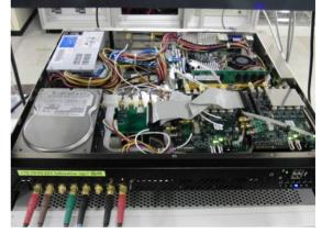
Figure 3: Photo of the digital filter (Dimtel Hadron BxB).
