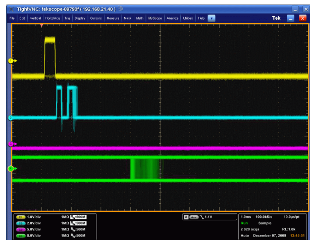
Figure 3: Measured data transmission time and jitter: 1ms after the clock trigger (upper, yellow line) all set points are delivered via reflective memory to the IOCs (middle, cyan line, 1ms/div). Without a sync event, 3ms later, with a jitter of 1ms, the last CAN object provides the set point to the power converter (bottom, green line).
