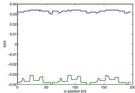
Figure 5: Calculated dynamic momentum aperture around the ring (including magnet errors and physical apertures).
