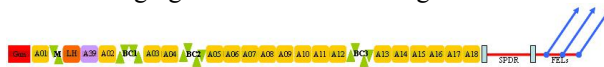
Figure 1: Schematic layout of the NLS FEL showing the location of gun, merger section (M), laser heater (LH), accelerating section (A01-A18), third harmonic cavity (A39), bunch compressors (BC1-3) and spreader section to the FELs.
