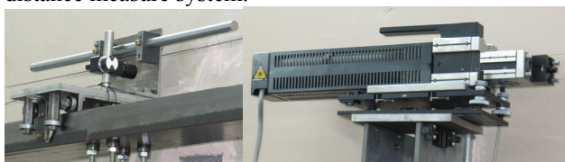
Figure 3: Laser and target of the distance measure system.
