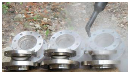
Figure 4: The chemical washing of injection channel elements.
