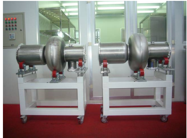
Figure 5: 500MHz niobium cavities after electric beam wilding. The cavity is based on KEKB type. The niobium material is from Ningxia, China.
